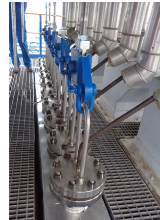
EARTH ® tubes in-tube thermocouples
